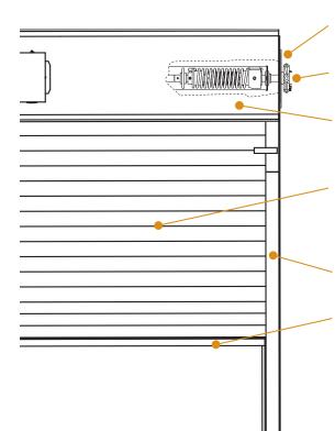
**BRACKETS** - Steel with powder coating to match curtin. Bolt to guide assembly and support counter-balance shaft and curtain.
