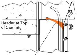
Lintel Seal Brush Contacting the Door Curtain
