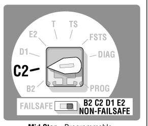
Mid Stop - Programmable **Open Override** - Available When Photo Eyes or Edge Sensor are triggered, the Door will Reverse and Fully Open.
