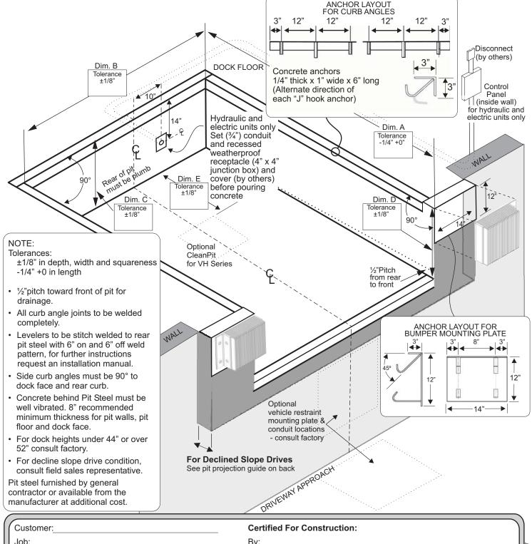
Pit dimensional tolerances are ±1/8" in depth, width and squareness, -1/4" +0 in length. POWERAMP/Systems, Inc. assume no liability for deviations beyond this tolerance.
