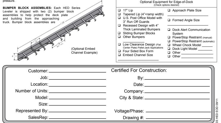
extra-heavy duty 4"x12"x13" constructed of formed steel and incorporate a full height internal gusset for extra support. All DLM bumper blocks feature 4" thick Tuf-Cord rubber bumper.
