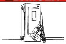
Hydraulic and electrical power must be OFF when servicing the equipment. For maximum protection, use an OSHA approved locking device to lock out all power sources. Only the person servicing the equipment should have the key to unlock the device.
